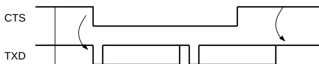
Figure 35-29. Transmitter Behavior when Operating with Hardware Handshaking
