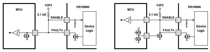
Figure 27. Methods For Operating in Retry Mode
