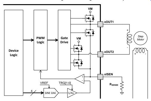
Figure 13. PWM Motor Driver Block Diagram
