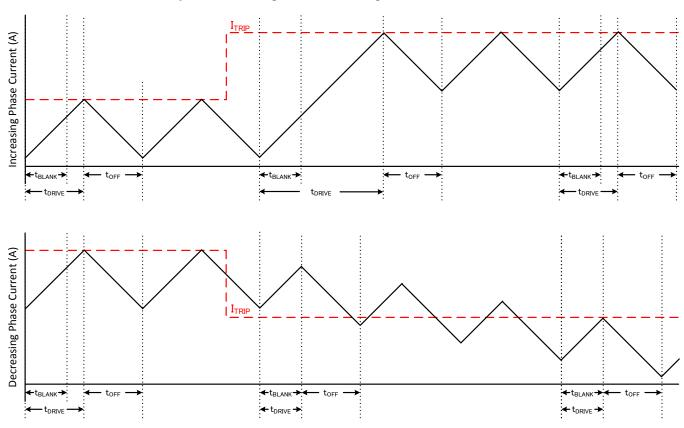
Figure 20. Fast/Fast Decay Mode
