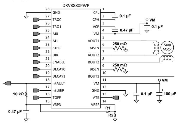
Figure 28. Typical Application Schematic
