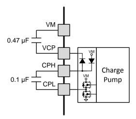
Figure 21. Charge Pump Diagram
