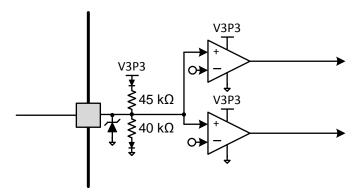
Figure 24. Tri-level Input Pin Diagram
