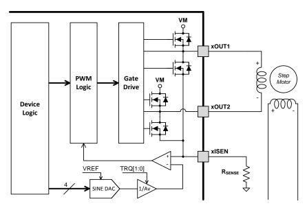
Figure 14. Current Regulation Block Diagram
