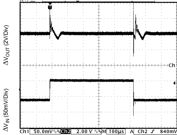
Figure 24. Line Transient Response
