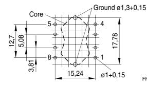
Hole arrangement View in mounting direction
