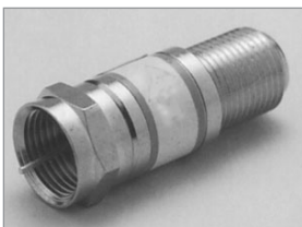
'F' Voltage Blocking Coupler Blocks DC and Low Frequency AC Power- Bandwidth: DC to 1 GHz, Return Loss 25db, (M) to (F).
