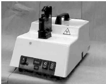
SDE Bench Terminator 1490076-2 (Customer Manual 409-10052)
