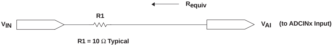
Figure 41. Typical ADC Input Pin Circuit
