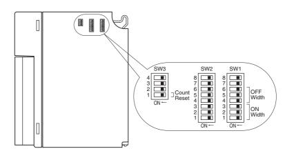
Count Reset SW must be turned off during operation.
