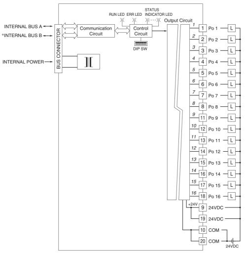
Numbers in italic indicate LED No.s assigned to the front panel LEDs.
