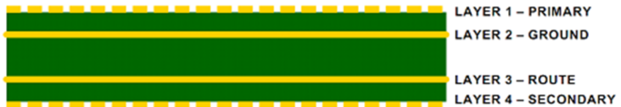
Figure 2. Four-Layer PCB Stackup
