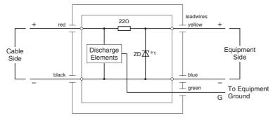
\*1. The zenor diode has polarity. Zero-cross signal cannot be connected.
