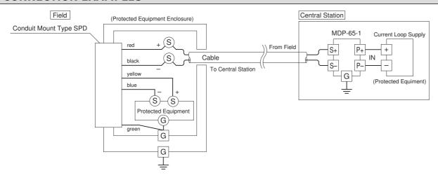
Connect the MD6P's green leadwire to the ground terminal inside the protected equipment enclosure to ground through the enclosure's outside ground terminal.
