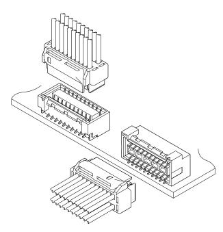
In order to correspond to the various highdensity PC board designing, this GHD connector is designed as 1.25 mm pitch double row type connector. Provide a full lineup of 10 to 40 circuits for top and side entry types.
