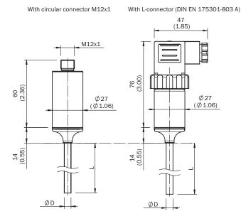
Process connection, weld-in thermowell
