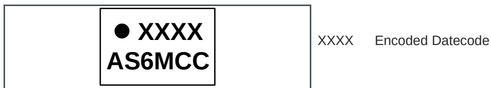
Figure 37: WLCSP Package Marking/Code
