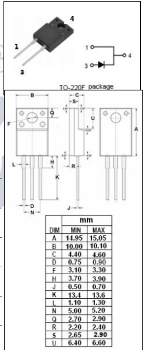
**Ultrafast Rectifier****BYV29X-600****THERMAL CHARACTERISTICS**
