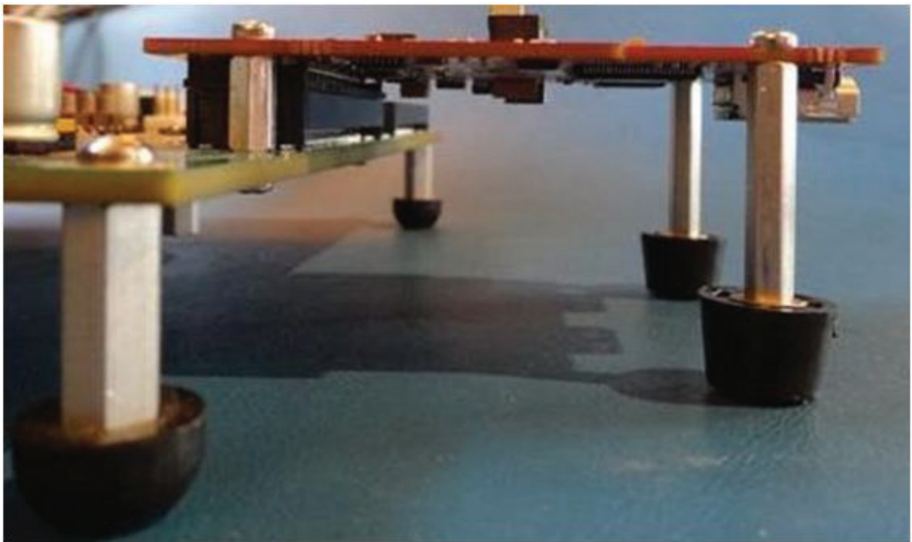
Figure 3-3: ZVIK FMC Mounting Hardware Detail
