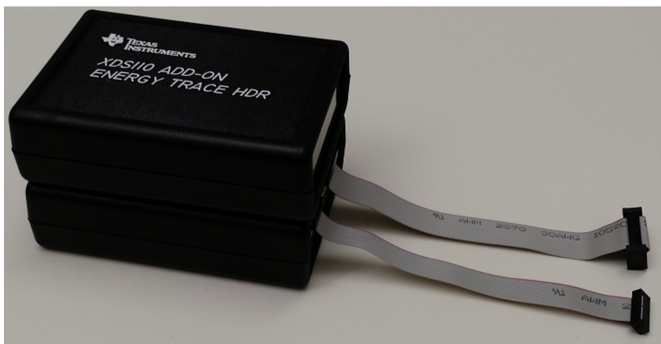
Figure 4. The XDS110 Probe and ETHDR System
