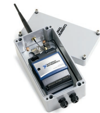
Figure 7. Outdoor Enclosure with NI WSN Measurement Node (not included)
