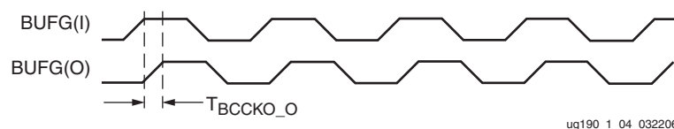
Figure 1-4: BUFG Timing Diagram
