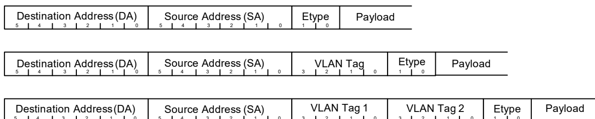
Figure 42 • Type II Ethernet Basic Frame Format
