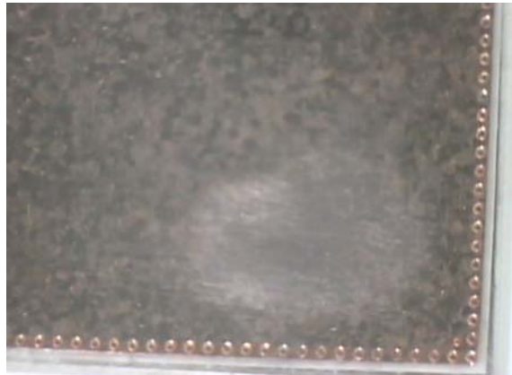
Fig. 5: Acceptable reworked MiniSKiiP bottom surface
