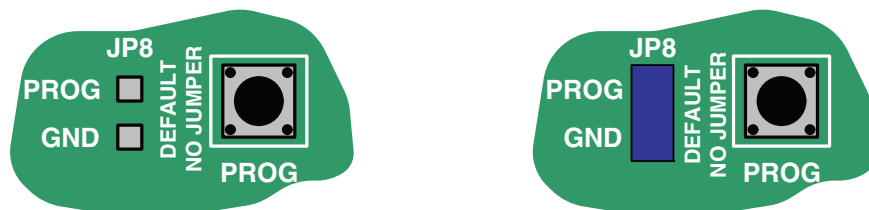
a) No Jumper: FPGA Operational (default)
