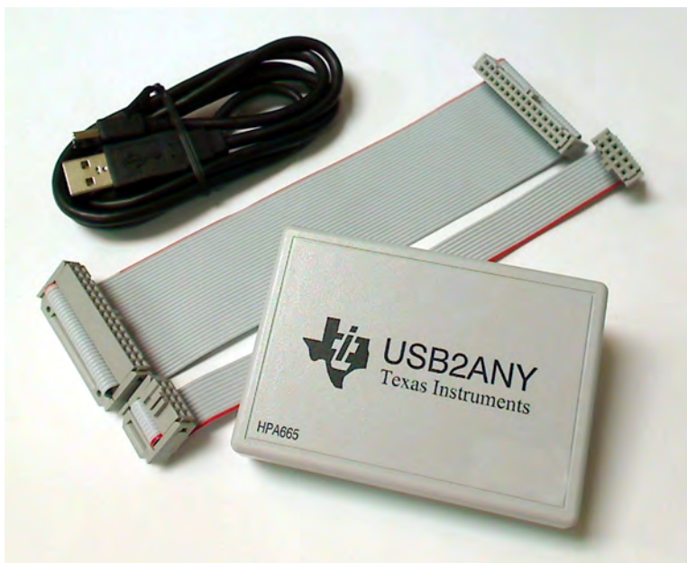
Figure 1. USB2ANY and the Supplied Cables
