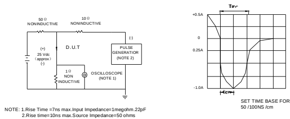
FIG.6-TEST CIRCUIT DIAGRAM AND REVERSE RECOVERY TIME CHARACTERISTIC
