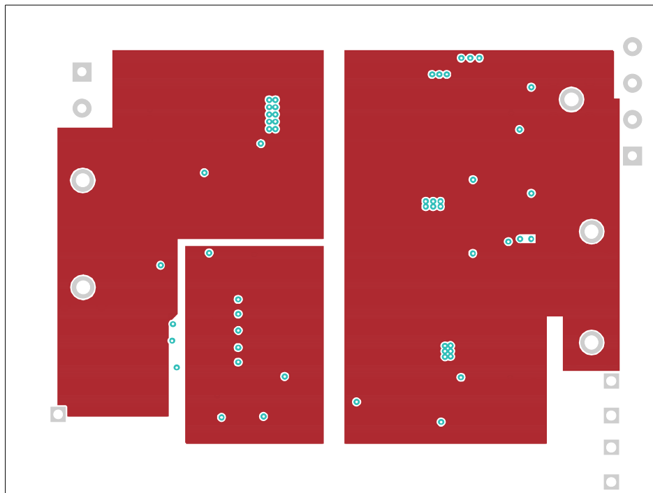
Figure 18. Internal Split Ground Plane
