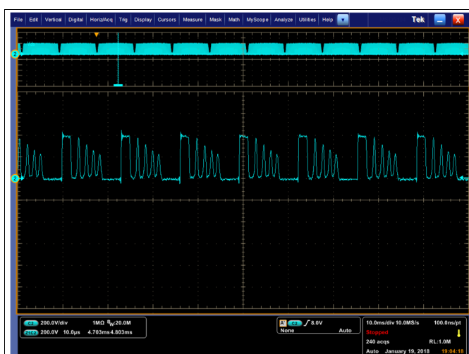
Figure 16. 85 VAC Valley Switching 50-mA Load
