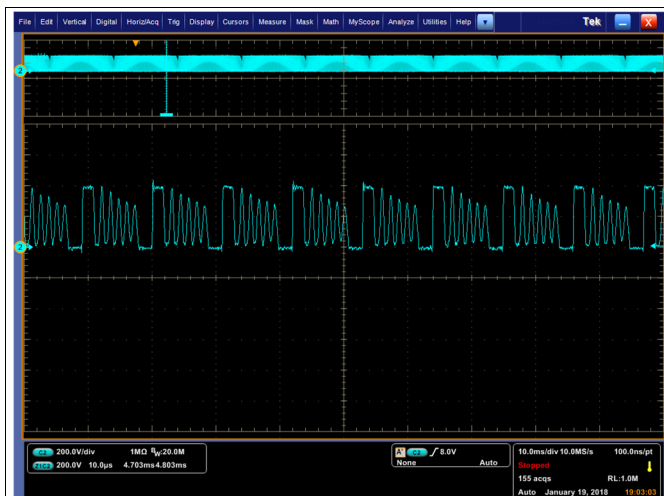
Figure 18. 230 VAC Valley Switching 100-mA Load
