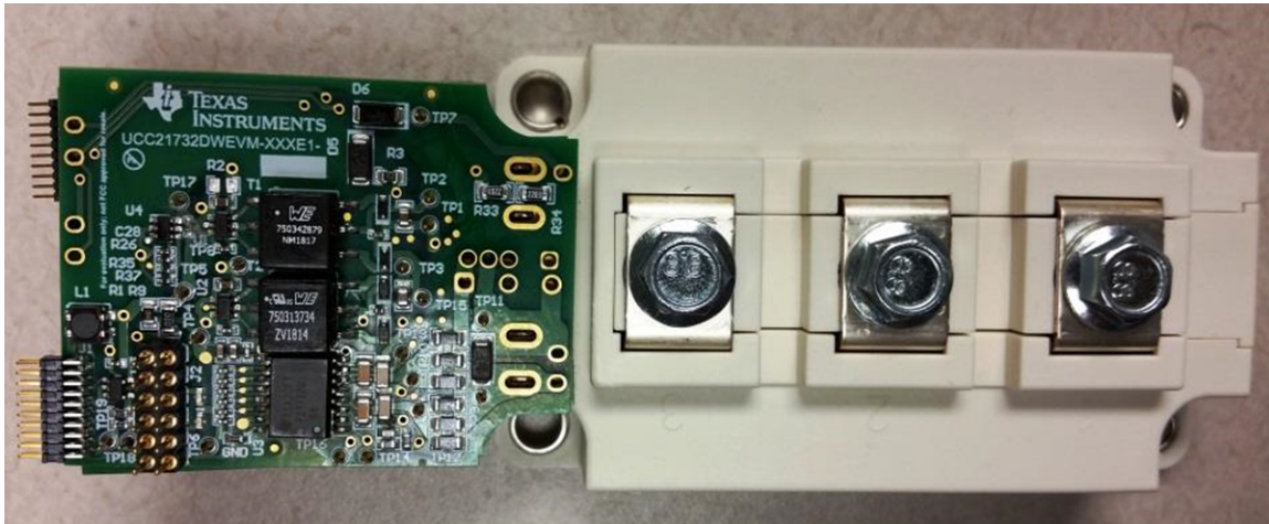
Figure 22. EVM Boards with Standard 106 mm Half-Bridge Module
