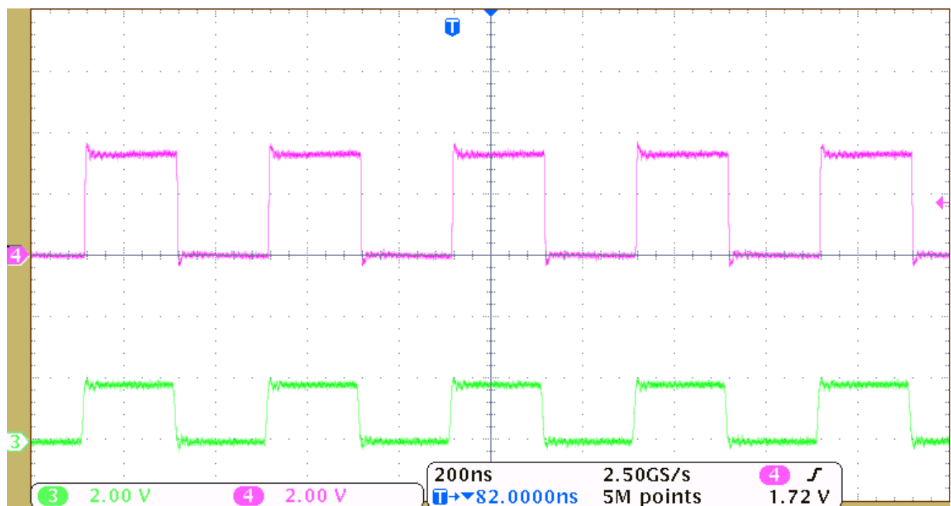
Figure 8. Level-Translation of a 2.5-MHz Signal
