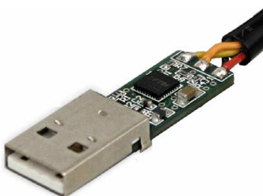
Figure 2 - Inside the USB 'A' connector on the TTL-232R.
