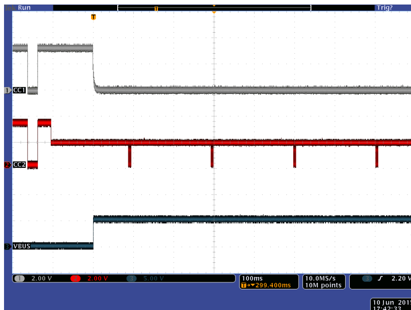
Figure 2. TPS65986 VBUS Voltage Transition
