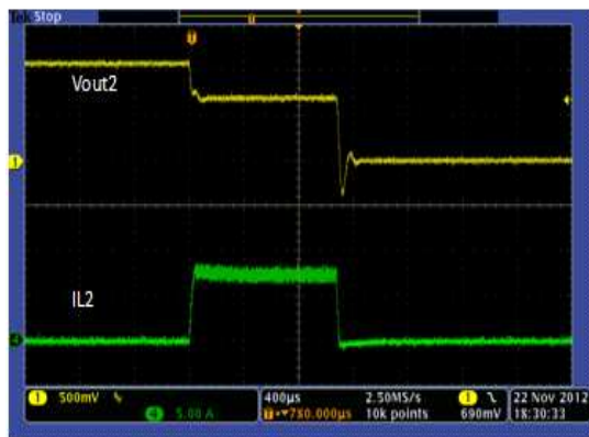
Figure 29. Over Current Protection, Buck 2
