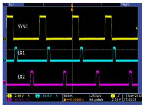
Figure 32. Synchronization at 500 kHz
