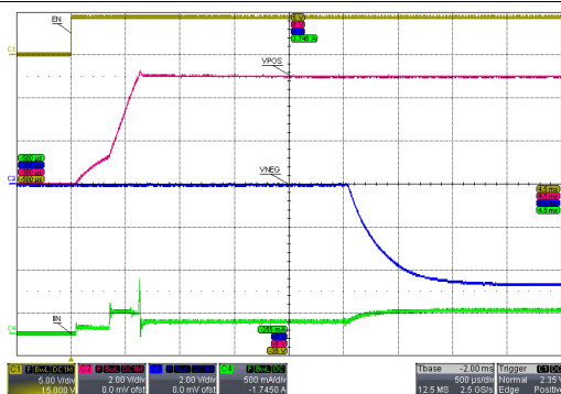
Figure 14. V_{NEG} Load Regulation
