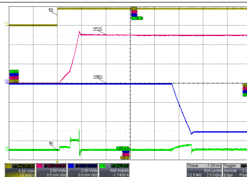
Figure 13. V_{POS} Load Regulation
