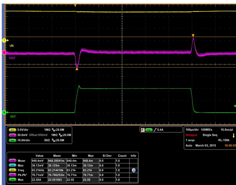
Figure 7. Transient Response of 0.95-V Output at 12 V_{IN} , Transient is 0 A to 20 A, 2.5 A/ \mu s
