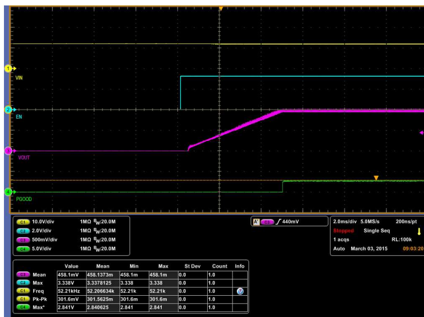
Figure 10. Start up from Control, 0.95-V Output at 12 V_{IN} , 20-A Output
