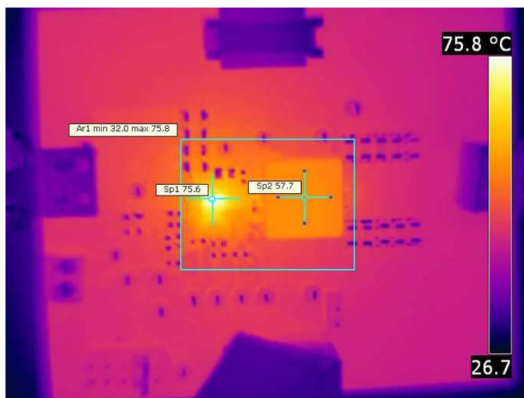
Figure 32. SP1: 75.6°C (TPS53515), SP2: 57.7 °C (Inductor)
