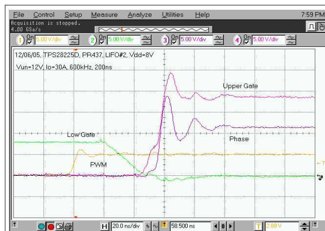
Figure 39. Phase Rising-Edge Switching Waveforms (20 ns/div) of the Power Stage in Figure 25
