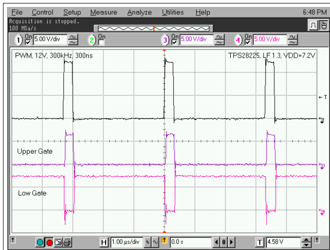
Figure 23. 12-V PWM Pulse at V_{DD} = 7.2 V
