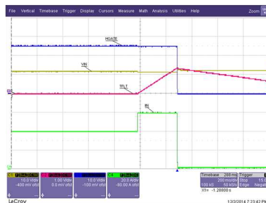
Figure 12. Load Step – 40 A to 60 A
