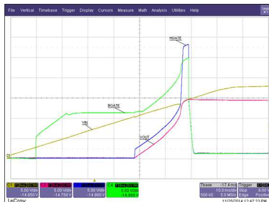
Figure 9. Under/Overvoltage With V_{IN} Rising
