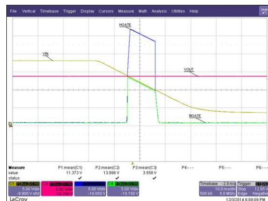
Figure 10. Under/Overvoltage With V_{IN} Falling
