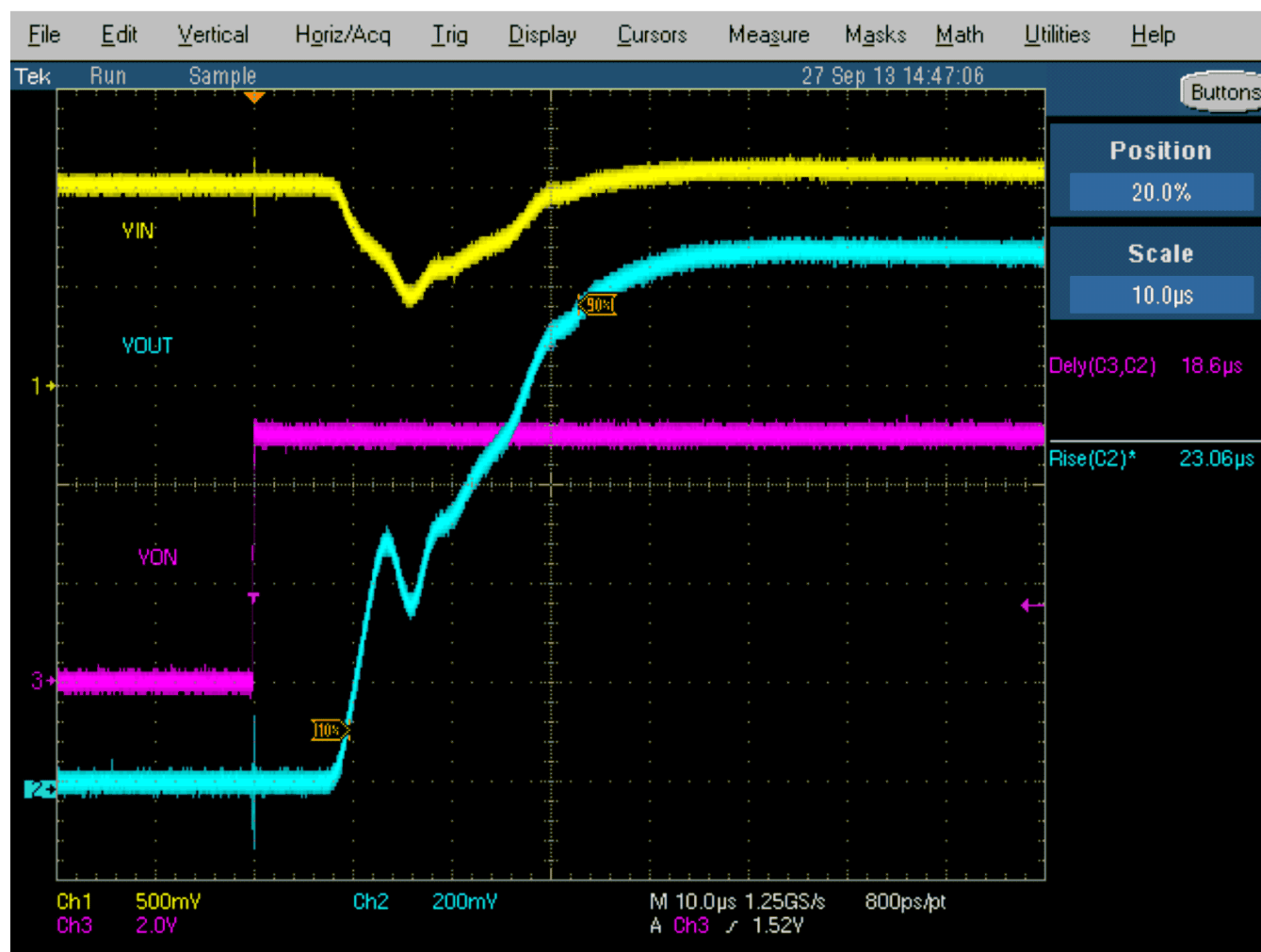
Figure 7. TPS22961 V_{out} t_R Example ( V_{BIAS} = 5V , V_{IN} = 1.05V , R_L = \text{Open} )
