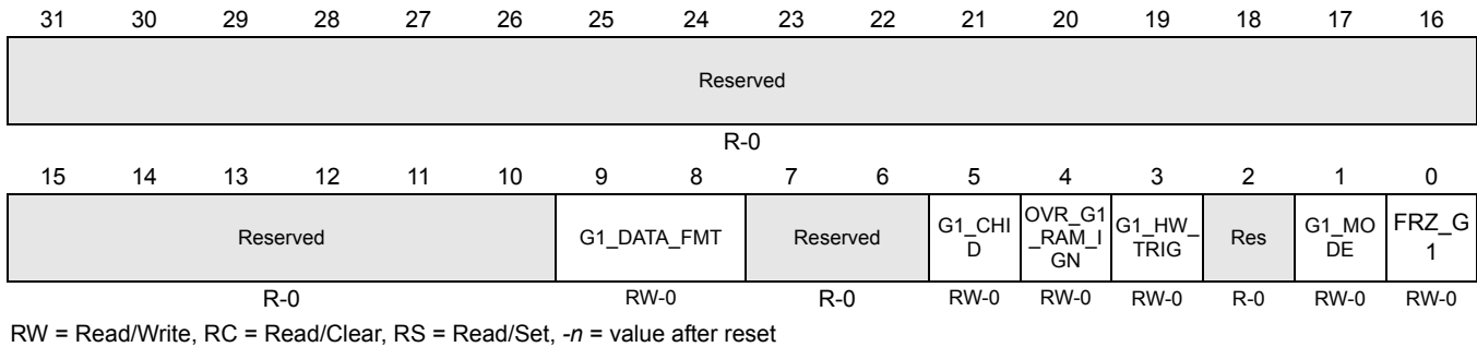
Figure 15-28. ADC Group1 Operating Mode Control Register (ADG1MODECR) [offset = 0x14]
