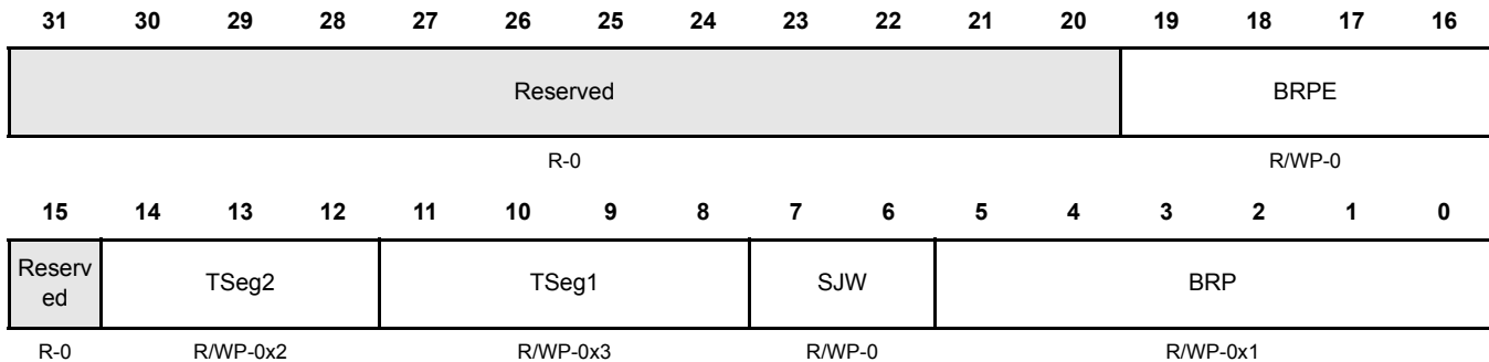
Figure 16-28. Bit Timing Register (DCAN BTR) [offset = 0x0C]
