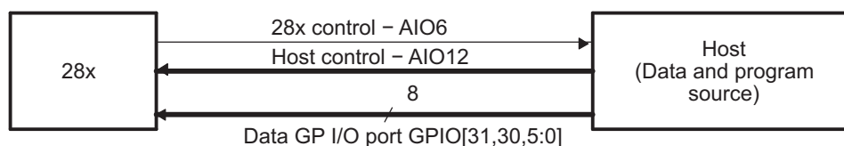
Figure 2-15. Overview of Parallel GPIO bootloader Operation
