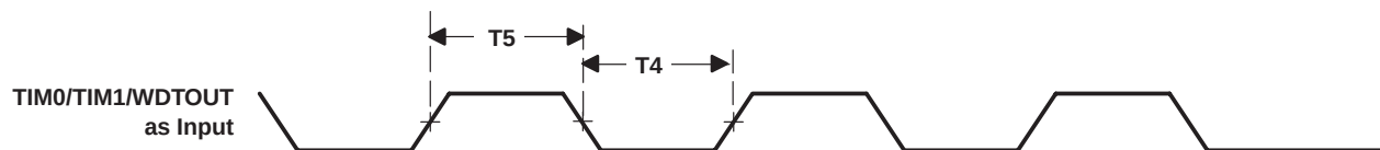
Figure 5–28. TIM0/TIM1/WDTOUT Timings When Configured as Timer Input Pins
