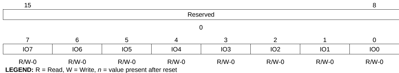
Figure 3-21. General-Purpose I/O Status Register (GPIOSR) [MMR Address 003Dh]
