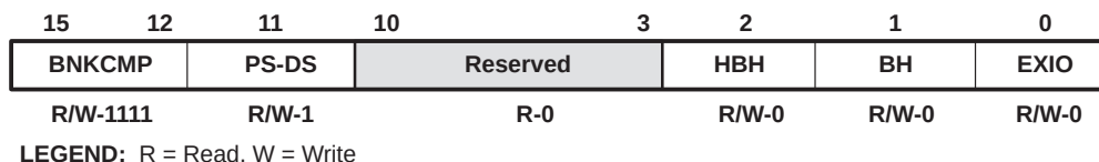
Figure 6. Bank-Switching Control Register (BSCR), MMR Address 0029h
