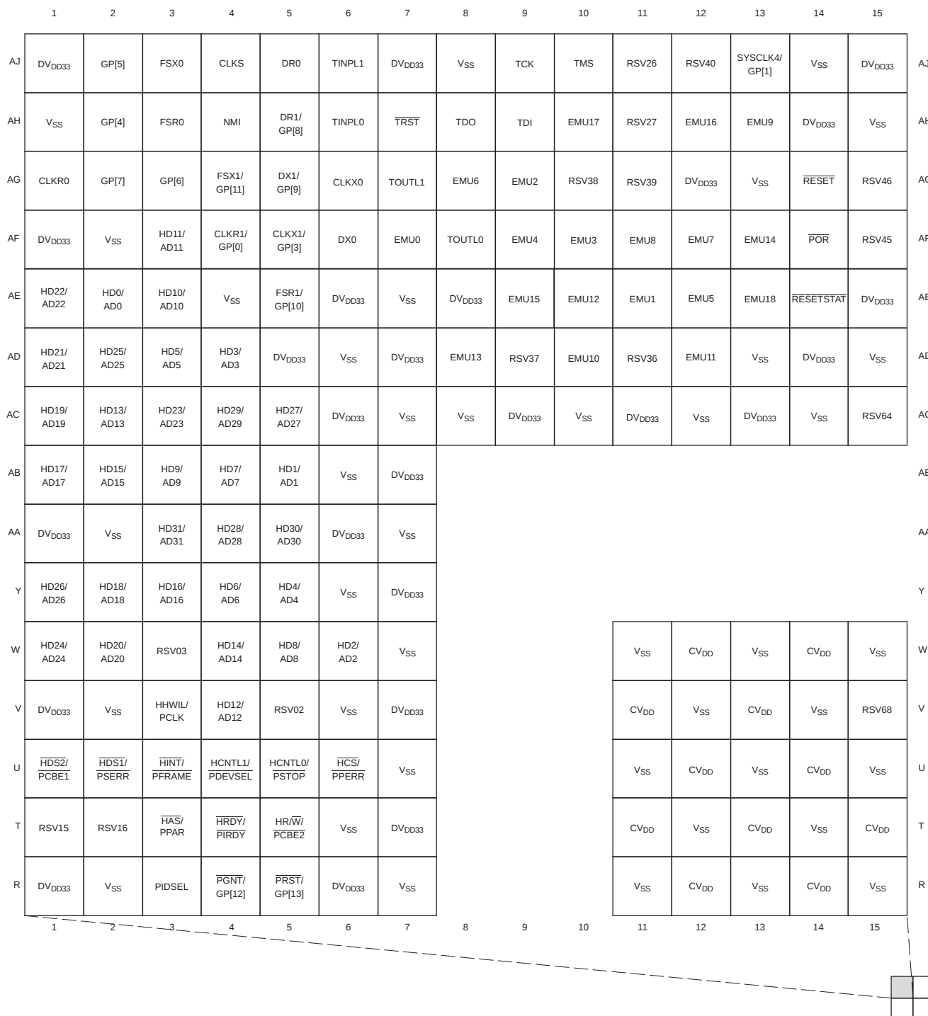
Figure 2-2. C6454 Pin Map (Bottom View) [Quadrant A]
