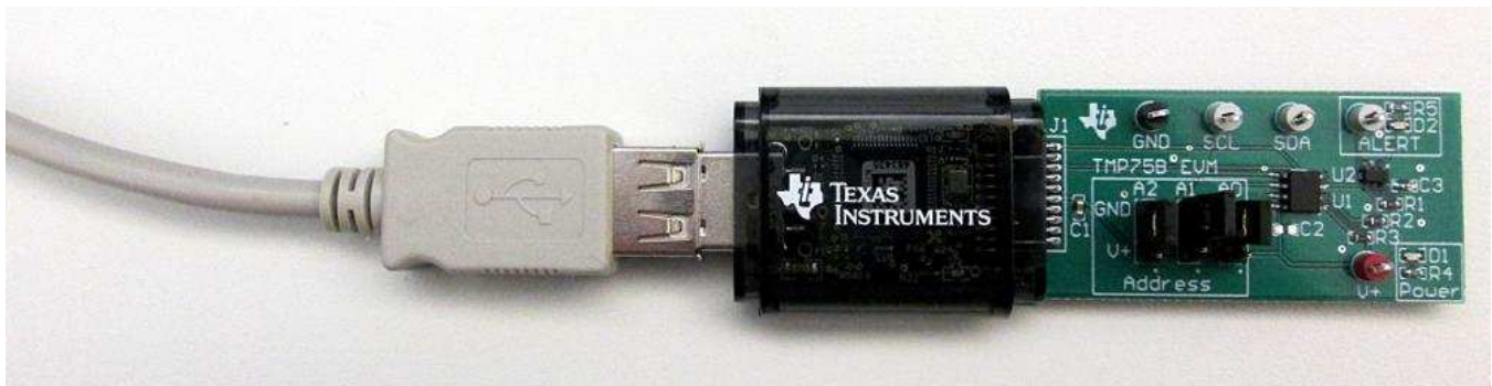
Figure 6. Typical Hardware Connection
