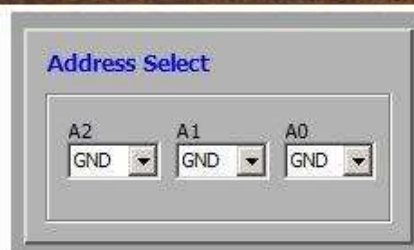
Figure 14. I²C Address Selection
