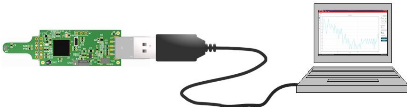
Figure 16. TMP117EVM Connection Diagram
