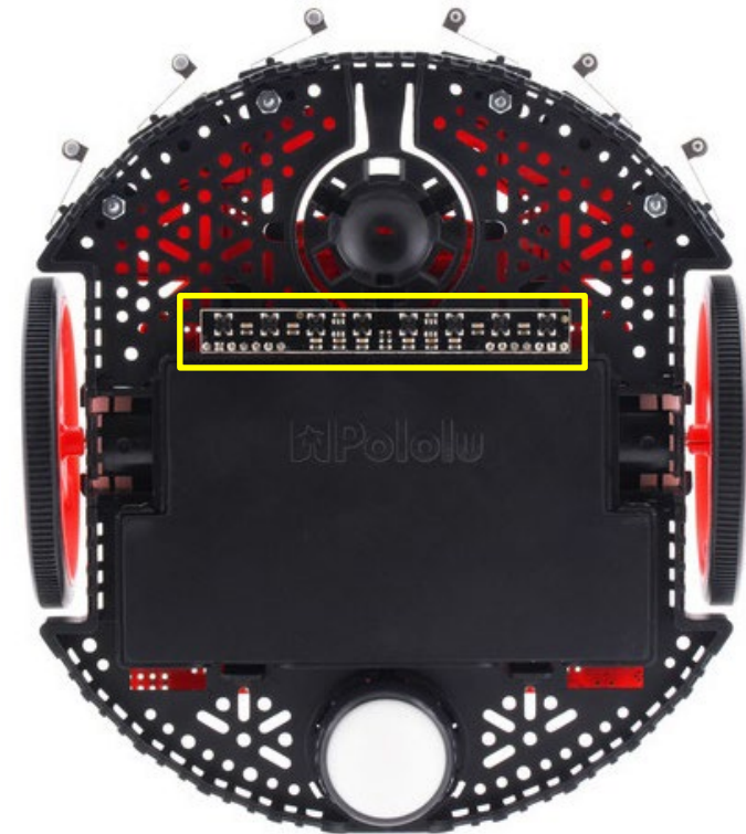
Figure 2. Remove the QTRX sensor, next to the battery compartment
