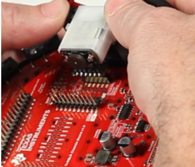
Figure 5. Pull the retaining tabs apart, just beyond white plastic motor casing
