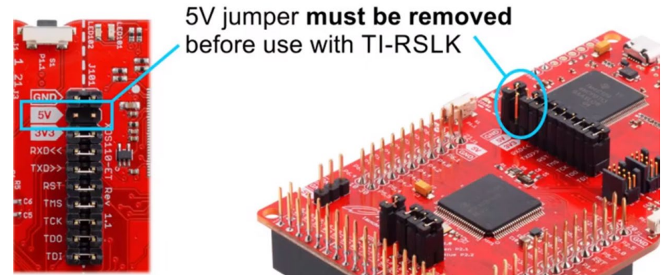
Figure 20. MSP432P401R LaunchPad with 5V jumper removed
