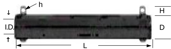
Standard Series T: Tubular design enables high power at low cost. Specialty high-temp flame resistant silicone ceramic coating holds wire securely against ceramic core providing optimum heat transfer and precision performance (enabling resistance tolerances to 0.1%).
