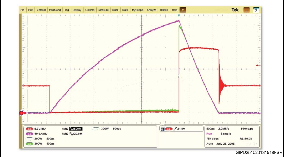
Figure 26. Unclamped inductive switching - experimental waveforms
