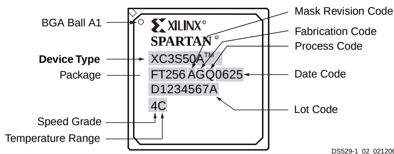
Figure 1-3: Spartan-3A FPGA BGA Package Marking Example
