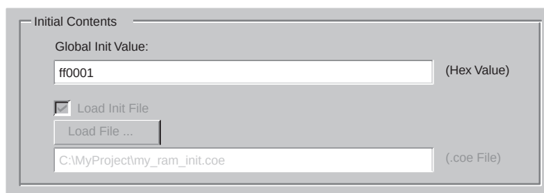
Figure 4-9: Specifying Initial Value for Block RAM Data Output Latches
