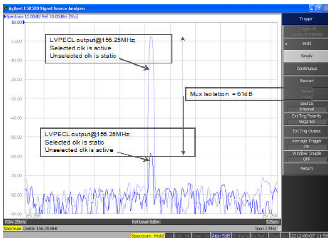
Figure 2.13. Input Mux Noise Isolation (Differential Input Clock, 44-QFN Package)
